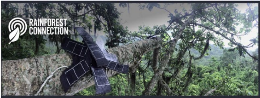
Figure 5-21. Example of installation made of solar panels and used mobile phones. Source: https://www.facebook.com/RainforestCx/
