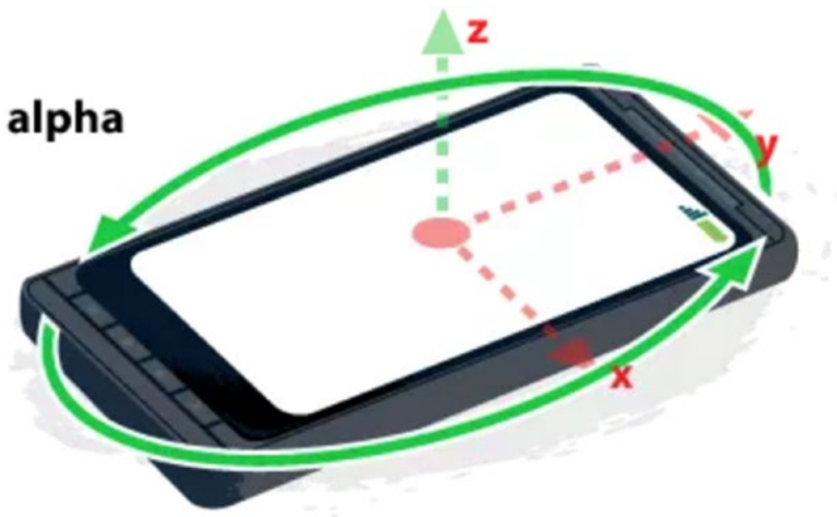
Figure 5-54. Gyroscope axes on mobile phone. Source: https://www.sitepoint.com/using-device-orientation-html5/
